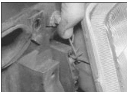
10.3 Releasing the headlight spring clips
