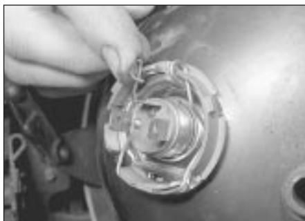
8.7a ... release the spring clips ...
