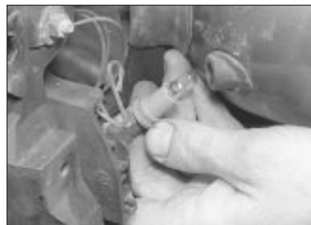
8.9 Removing the front parking light bulbholder
