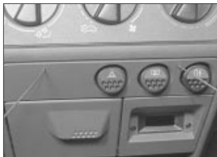
4.13b Insert lengths of rod into the special holes . . .
