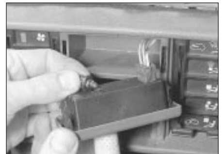
9.11 Removing digital clock illumination light bulb
