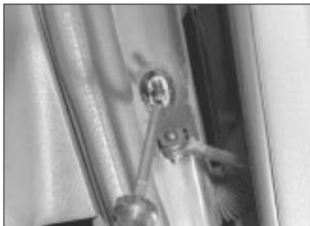
4.21 Removing a courtesy light switch
