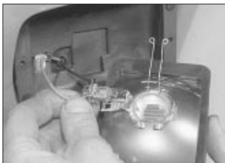
8.16 ... then release the spring clips and remove the bulb assembly
