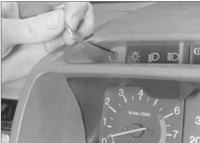
5.2 Removing the instrument panel upper ...
