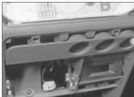
4.13c . . . and withdraw the switch panel surround
