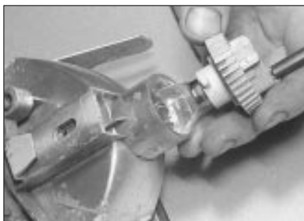
8.10 Remove the front direction indicator light bulbholder ...
