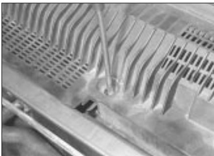
15.3 Removing the air intake grille screws
