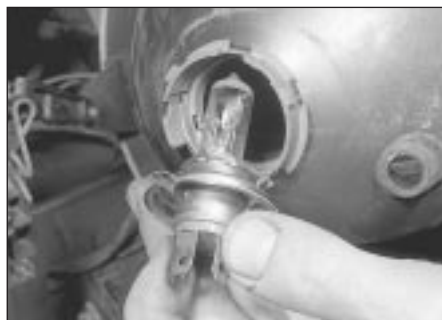
8.7b ... and withdraw the headlight bulb
