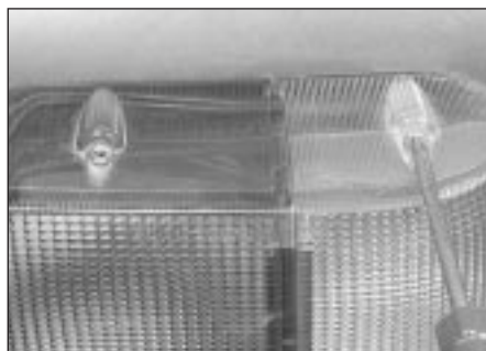
8.18a Remove the rear light cluster screws ...
