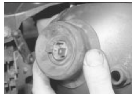
8.6 . . . remove the rubber cover . . .
