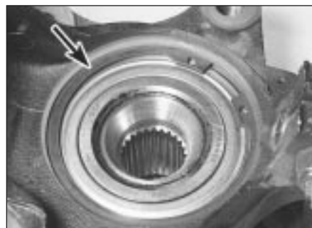
3.3 Front hub bearing retaining circlip (arrowed)
