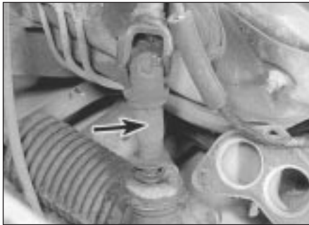
14.7 Steering column intermediate shaft (arrowed)
