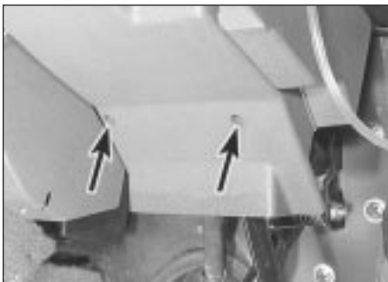
14.2 Steering column lower trim panel screws (arrowed)
