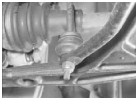
7.9 Anti-roll bar link arm bottom mounting on GTI models
