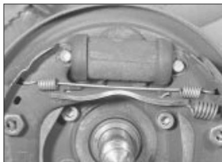
5.4 Upper return spring location (DBA Bendix type)
