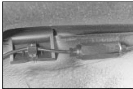
13.7 Rear brake compensator fitted to 1.9 GTI models
