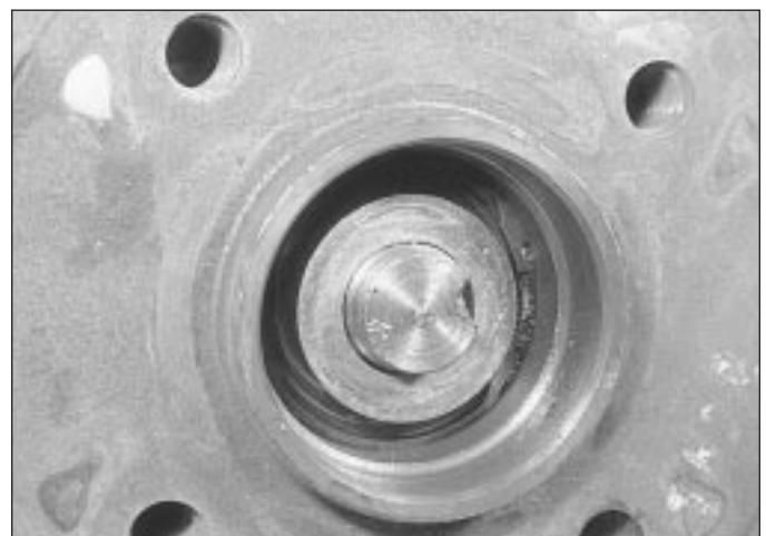
11.2b . . . and remove the washer
