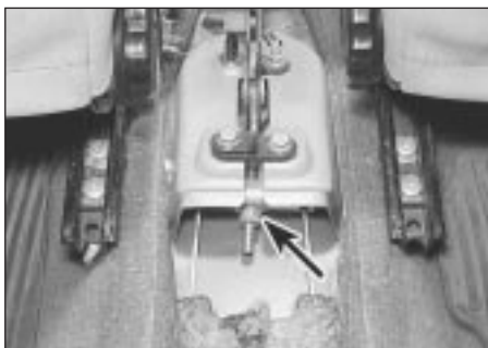
15.5 Handbrake adjustment nut and locknut (arrowed)
