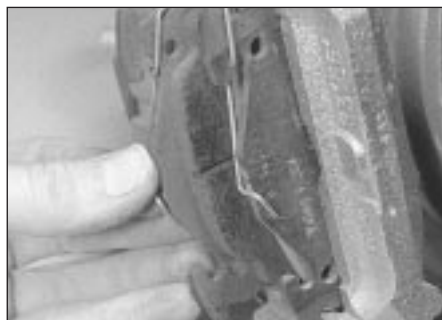
6.3 Removing the rear brake pads
