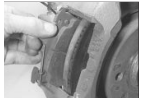
4.6 Removing the inner pad (DBA Bendix caliper)
