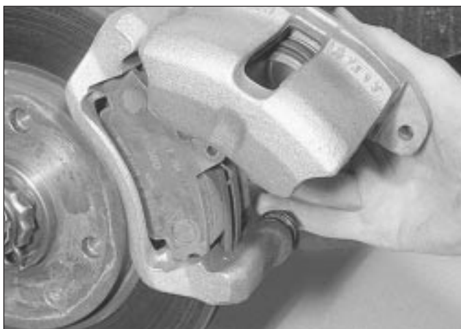
4.20a Swivel the caliper upwards . . .
