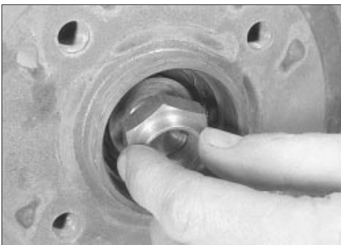
11.2a Unscrew the rear hub nut . . .
