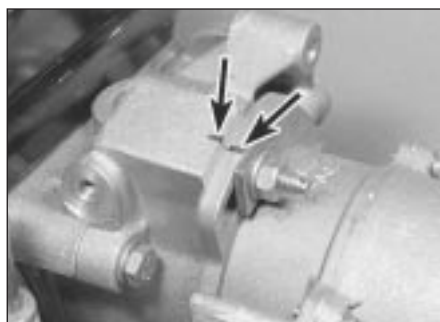
4.17 Mark the distributor and housing . . .
