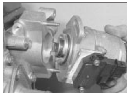
4.18 . . . then remove the distributor
