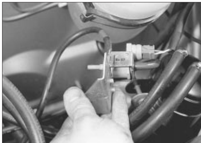
8.7b . . . and withdraw the solenoid bracket
