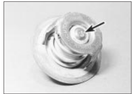
4.9 Thermostat temperature rating (arrowed) stamped on base
