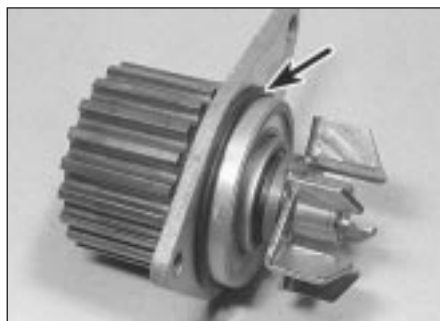
8.18b . . . then recover the O-ring seal (arrowed)
