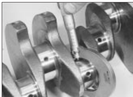
8.40 Measuring a crankshaft big-end journal diameter
