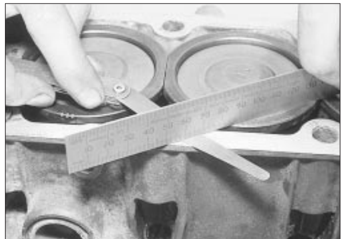
9.24 Measuring cylinder liner protrusion
