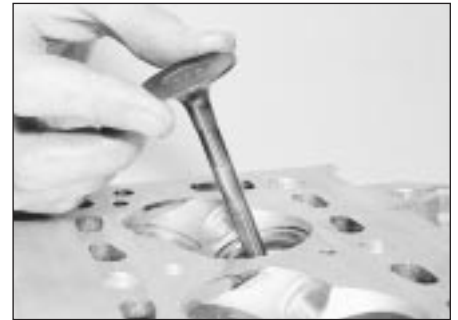
6.6 Withdraw the valve through the combustion chamber
