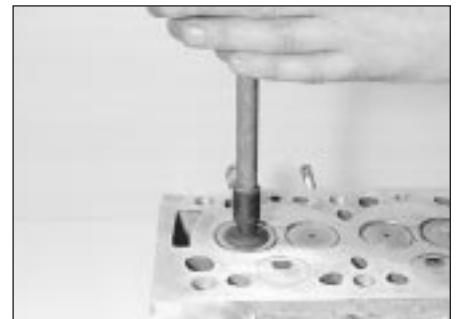
6.21 Grinding-in a valve
