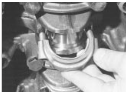
7.11 Removing a big-end bearing cap and shell
