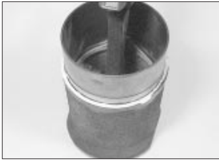
9.11 Cylinder liner with paper base seal
