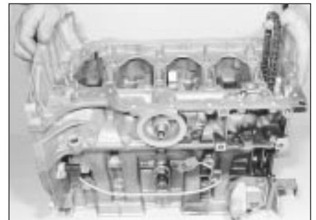
13.74 . . . then lower the main bearing ladder into position
