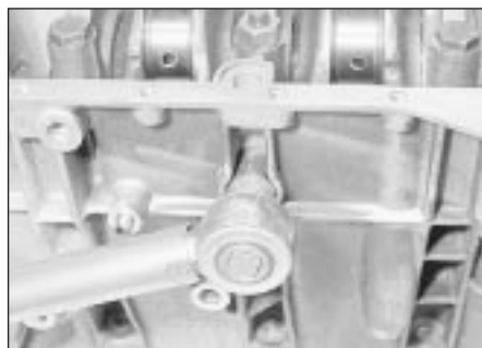
13.60 Refit and tighten the centre main bearing side bolts
