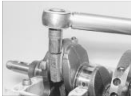
14.22 Tightening a big-end bearing cap nut using a torque wrench . . .
