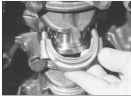
10.5 Removing a big-end bearing cap and shell
