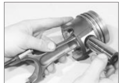
13.15b . . . and withdraw the gudgeon pin
