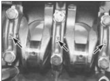
11.17 Main bearing cap identification markings (arrowed)
