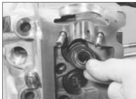
7.4c Remove the spring retainer . . .
