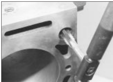
12.9 Cleaning a cylinder block threaded hole using a suitable tap
