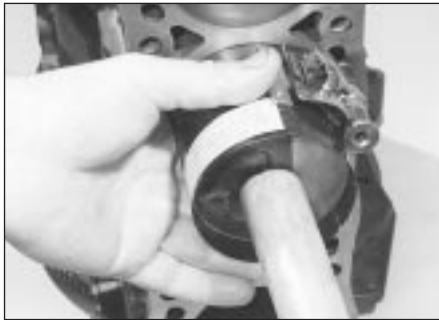
19.19 Tap the piston into the bore using a hammer handle
