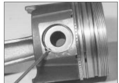
13.15a On 16-valve engines, prise out the circlip . . .
