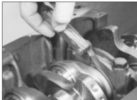
14.3 Checking crankshaft endfloat using feeler gauges
