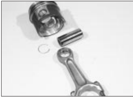
13.15c Piston and connecting rod components
