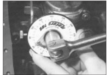
19.22b . . . then through the angle specified for stage 3
