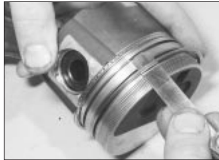
13.2 Removing a piston ring with the aid of a feeler gauge
