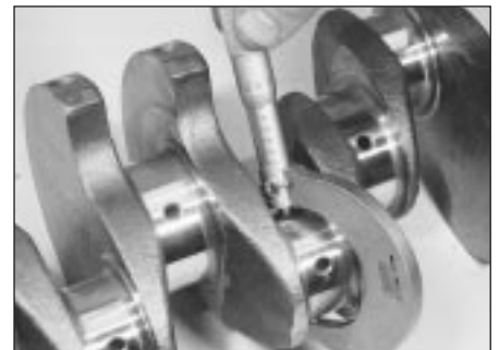
14.10 Measuring a crankshaft big-end journal diameter
