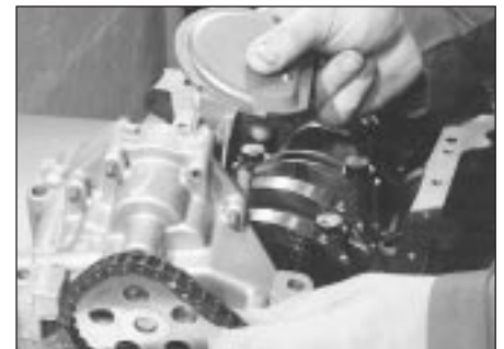
10.3 Removing the oil pump
