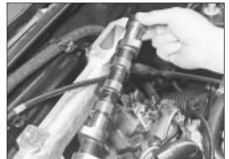
7.9 Lift the camshaft from the cylinder head
