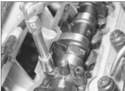
7.7 Progressively unscrew the camshaft bearing cap nuts . . .
