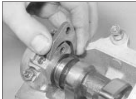
10.38b . . . and remove the camshaft thrust fork from the bearing cap
