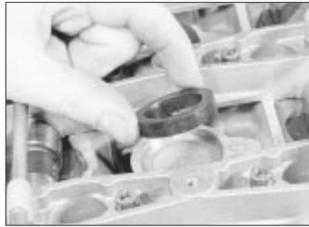
4.32 Fitting a spark plug hole oil seal
