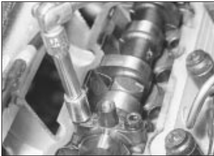
10.31 Working as described in the text, unscrew the retaining nuts . . .
