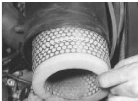
26.2 . . . and remove the cover and filter element
