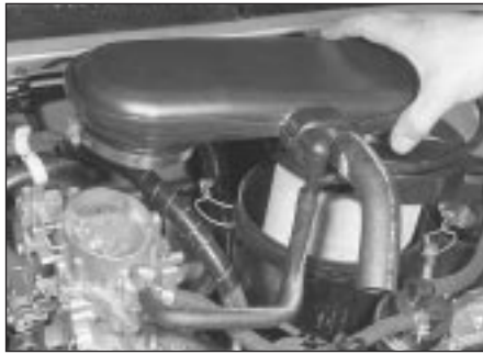
26.5c . . . then lift off the top, or end cover
