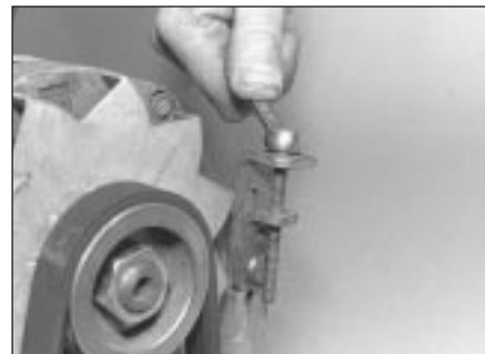
9.9 Slackening the alternator adjuster bolt to release the auxiliary drivebelt
