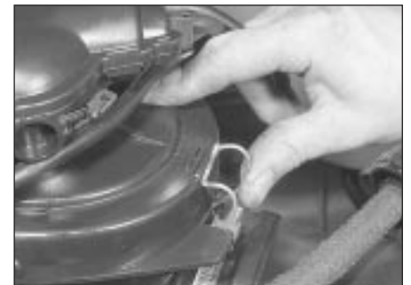
26.5b . . . or release the spring clips . . .
