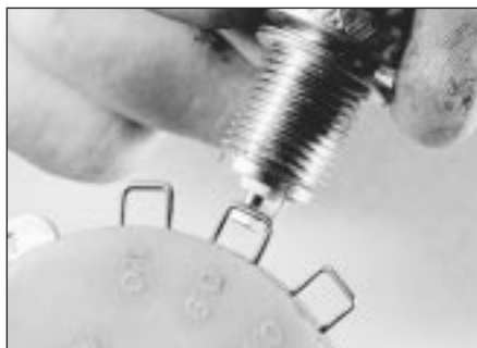
7.10 Measuring the spark plug gap with a wire gauge
